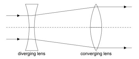
The rays emerge parallel from the converging lens. Determine the distance between the two lenses.
