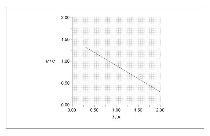
Using the graph, determine the best estimate of the internal resistance of the cell. [3]
