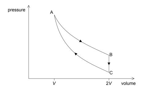
At A the pressure of the gas is  $4.00 \times 10^6$  Pa, the temperature is 612 K and the volume is  $1.50 \times 10^{-4}$  m<sup>3</sup>. The work done by the gas during the isothermal expansion is 416 J.
