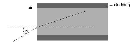
The ray makes an angle A with the normal at the air—core boundary. The refractive index of the core is 1.52 and that of the cladding is 1.48.
